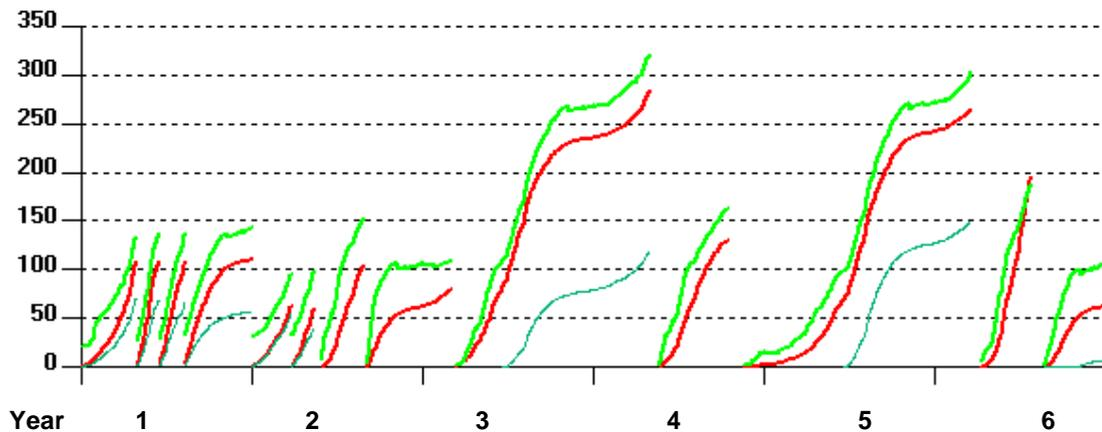
Figure 3: Cumulative nitrogen availability (green line), crop uptake (red line) and nitrogen fixation (turquoise). Y-axis:  $\text{kg N ha}^{-1}$
