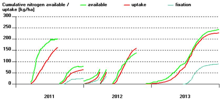
Figure 8: Cumulative nitrogen availability (green line), crop uptake (red line) and nitrogen fixation (turquoise). Y-axis:  $\text{kg N ha}^{-1}$
